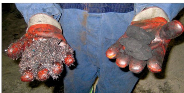
One of the two main lithium-ion battery recycling processes used today involves pulverizing the modules and then using a screen to separate components. For Tesla car batteries, this process gives a copper cobalt fluff (left) that is sold to recover useful metals, and a slurry that is processed into a cobalt filter cake (right) that can be reused in appliance coatings. Credit: Tesla Motors.
