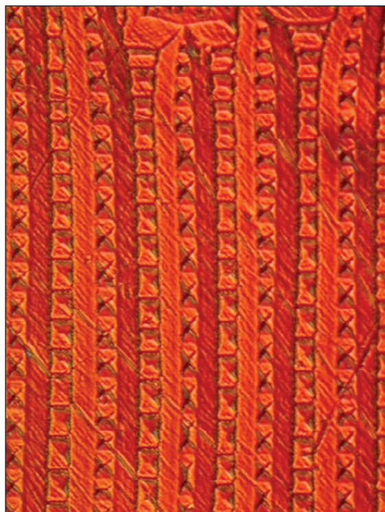
Cellular domains in non-Joulian Fe-Ga magnets. Figure courtesy of Harsh Deep Chopra/Temple University.
