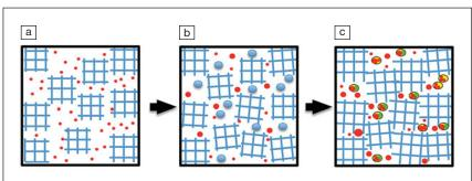
The formation of lead nanospheres in zircon: (a) Metamict zircon with inclusions of incompatible elements like Pb and Si; (b) inclusions grow in size due to Ostwald ripening; and (c) Pb precipitates out of melt inclusions forming nanospheres. Reprinted with permission from *Proc. Natl. Acad. Sci. U.S.A.* **112** (16) (2015), DOI: 10.1073/pnas.1415264112; p. 4958. © 2015 National Academy of Sciences.
