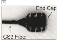
(a) Schematic of the multicore-shell printing process; (b) schematic of the sensor assembly process; and (c) sensor integration with textiles through sewing. Reprinted with permission from Adv. Mater. 27 (2015), DOI: 10.1002/ adma.201500072. © 2015 Wiley.
