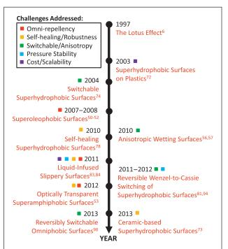
Figure 4. Timeline of key materials innovations and developments in bioinspired liquid-repellent surfaces in the past decade (2003-2013). 6,50-53,56,57,72-74,78,81,83,84,90,94 Note that this timeline only covers material development and does not include the key fundamental theoretical/computational/experimental discoveries during the period. Readers are referred to recent reviews by Quéré, <sup>4</sup> Marmur, <sup>95</sup> Nosonovsky and Bhushan, <sup>96</sup> and Bormashenko.97
