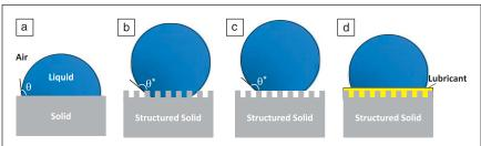
Figure 3. Wetting on smooth and structured surfaces. A liquid droplet sitting on (a) a smooth surface with an intrinsic contact angle,  $\theta$ ; (b) a textured surface that is completely wetted by the liquid, known as a Wenzel state droplet; (c) a textured surface with trapped air pockets, known as a Cassie state droplet; and (d) a textured surface that is infused with an immiscible lubricating fluid (or slippery liquid-infused porous surfaces). Note:  $\theta^*$ , apparent contact angle.
