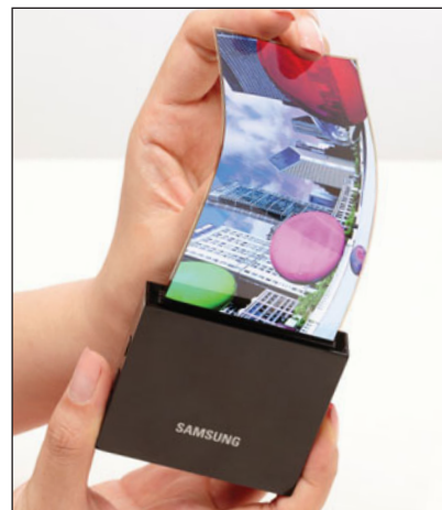
Samsung's prototype of a flexible organic light-emitting diode display called “YOUM.” Courtesy Samsung Electronics Co., Ltd.
