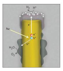
This cross-sectional schematic of an individual plasmonic solar water splitter unit consists of a gold nanorod, the TiO<sub>2</sub> cap (decorated with platinum nanoparticles)— which functions as the H<sub>2</sub> evolution cata-lyst—and the Co-based O<sub>2</sub> evolution catalyst deposited on the lower portion of the gold nanorod. Reproduced with permission from *Nature Nanotech.* **8** (2013), DOI: 10.1038/ NNANO.2013.18; p. 247. © 2013 Macmillan Publishers Ltd.
