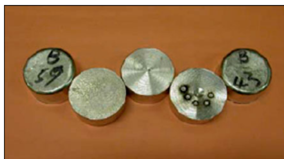
Figure 3. Disks of Standard Reference Material (SRM) 1728 Tin Alloy (Sn–3Cu–0.5Ag), a lead-free solder composition, showing various stages in manufacturing and testing. The alloy was created using a semi-chill casting process to ensure homogeneity of the disks to a depth of at least 10 mm. The SRM provides values for bulk composition of a number of elements, including chromium, cadmium, mercury, and lead, which are restricted in products around the world for environmental and health reasons. 33
