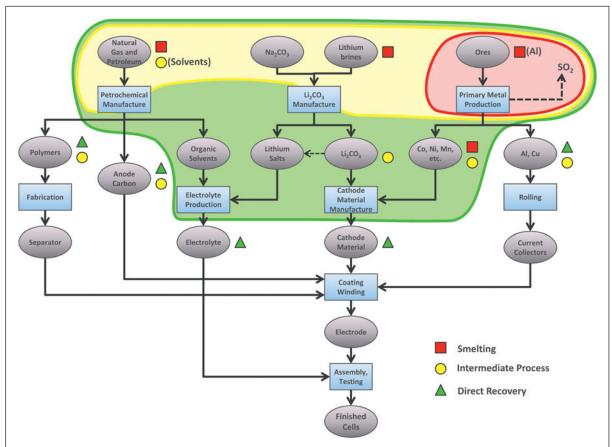
Figure 3. Schematic flow chart for the production of lithium-ion cell materials. where purple ovals and light blue rectangles represent component materials and process steps, respectively. 10 The red, yellow, and green symbols next to various components indicate where new materials can be replaced by smelting, by the intermediate process, and by direct recovery, respectively, and the corresponding shaded outlines encompass the process steps that are avoided by each of these alternative flows.
