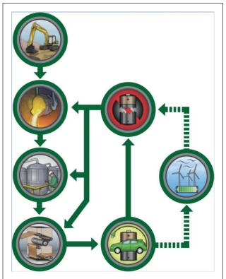
Figure 1. Schematic of battery recycling to different manufacturing stages: This figure depicts mining of ore, primary processing, chemical conversions, and fabrication into a battery. The finished battery is then used in a vehicle and is recycled back to one of the manufacturing steps, possibly after being reused to store energy for an electric utility.
