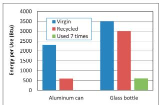
Figure 2. Energy per use for 12-oz. single-serving beverage containers. To compare different options, the total energy for original manufacturing and all processes involved in recycling or reuse is averaged over the number of uses.
