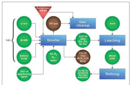
Figure 4. Flow chart for the recycling of lithium-ion batteries by smelting (data courtesy of Umicore). The blue rectangles indicate the steps in the process, whereas the green and brown circles represent material inputs and outputs, respectively. The red triangle shows an energy input of 800 MJ.
