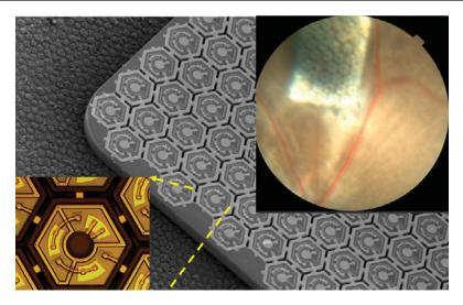
Subretinal photodiode array with triple-diode pixels arranged in a hexagonal pattern. Pixels of 70  $\mu$ m and 140  $\mu$ m in size were made. Left inset: Central electrodes are surrounded by three diodes connected in series, and by the common return electrode. Right inset: The subretinal implant.
