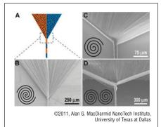
knitted, and braided into a variety of structures. In one example, as reported in Physicsworld.com, superconducting yarn was made by biscrolling a mixture of magnesium and boron powders (up to 99 wt%) as the guest on CNT sheets, and then thermally annealing the
