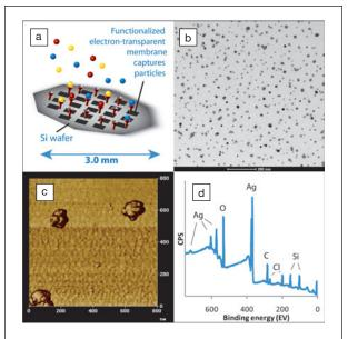
Figure 1. Dune Sciences' SMART grids products capture and immobilize materials for nanoscale characterization using a wide range of analytical tools: (a) SMART grids; (b) transmission electron micrograph of silver nanoparticles (AgNPs) captured on NanoPLUS<sup>™</sup> grids; (c) atomic force micrograph of degraded AgNPs on NanoPLUS grid; and (d) x-ray photoelectron spectroscopy results of Ag NPs on NanoPLUS grids.
