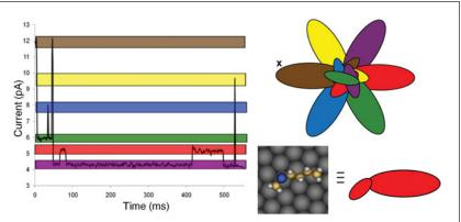
An example of a current versus time spectrum that provides a way of monitoring the rotation of butyl methyl sulfide between six different orientations shown in the schematic (top right). A model of the molecule on the Cu(111) surface is shown at bottom right. Reproduced with permission from Nature Nanotech. 6 (2011), DOI: 10.1038/NNANO.2011.142; p. 625. © 2011 Macmillan Publishers.
