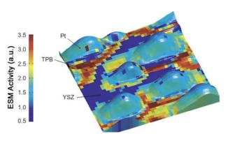
Map of electrochemical activity is overlaid onto the topography of Pt catalyst dots deposited on a YSZ surface. TPB indicates a triple-phase boundary where the catalyst electrode is in contact with both the reactants and electrolyte. Reproduced with permission from *Nature Chem.* (DOI: 10.1038/NCHEM.1112; p. 707). © 2011 Macmillan Publishers Ltd.
