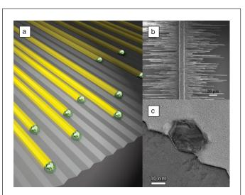
(a) Illustration of nanowires growing along nanogrooves; (b) top view of the nanowires by scanning electron microscopy; and (c) cross-section view of a nanowire along a V-shaped nanogroove by transmission electron microscopy. *Image credit*: Ernesto Joselevich.
