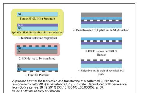
to transfer electronic and photonic devices without compromising structural integrity and functionality. The researchers describe their fabrication protocols in the January 1st issue of *Optics Letters* (DOI:10.1364/
