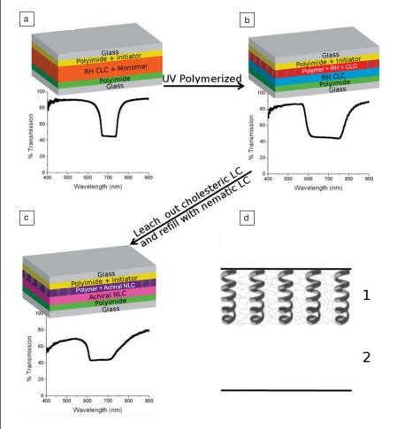
Figure 1. (a-c) Fabrication steps are represented schematically, along with corresponding transmission spectra; (d) a cartoon illustrating the two distinct regions in the cell separated across the z-direction. RH CLC is right-handed cholesteric liquid crystal; NLC is nematic LC. Reproduced with permission from Chemical Communications 47 (2011) DOI: 10.1039/c0cc02215b; p. 505. © 2011 Royal Society of Chemistry.
