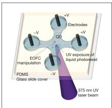
A microfluidic device for precisely positioning quantum dots on a surface using electroosmotic flow control (EOFC). A UV laser is used to polymerize the fluid and trap individual quantum dots in place. Reproduced with permission from Nano Lett. 10 (11) (2010) DOI: 10.1021/nl1029557; p. 4673. © 2010 American Chemical Society.
