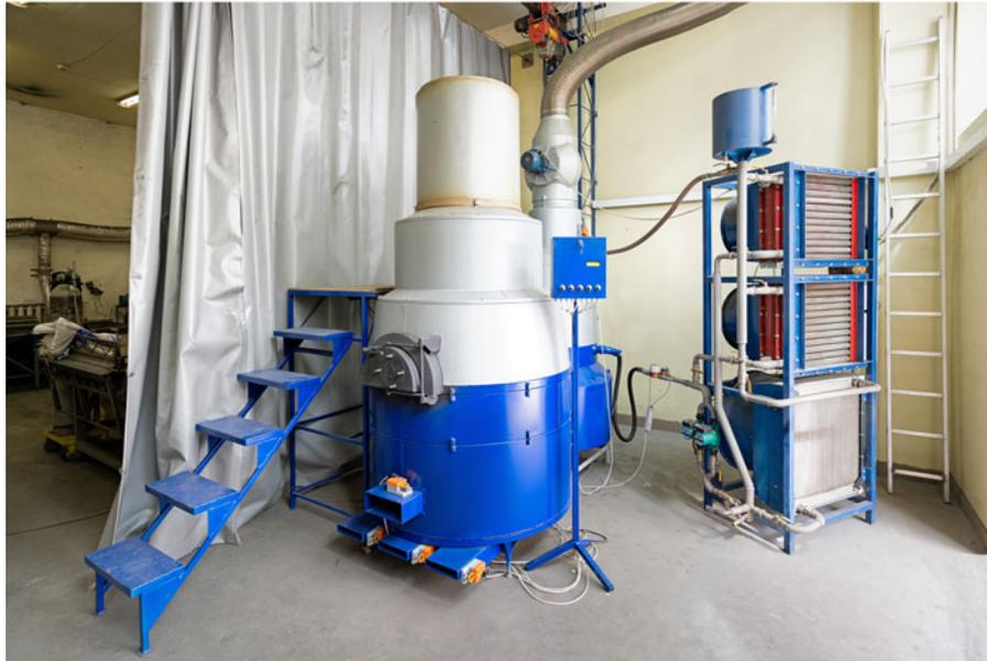
**Figure 1.** Our gasifiers of 2016 (a, which recycles 30 kg/h of waste) and of 2018 (b, which recycles 80 kg/h of waste).
