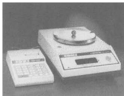
prevent incorrect data from being displayed should either of these problems occur. When combined with an application keyboard, dedicated printer or RS 232 interface, the balance's capabilities can be expanded to include statistical calculation. Hook-up to the RS 232 or application keyboard permits two-way communication between balance and PC or other external device. PTX-Pentronix, Inc., 1737 Cicotte Lincoln Park, MI 38146-1304; (313) 388-3100.
