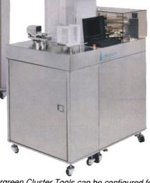
Polypropylene chambers are available for acid processing. In addition, this Model 50 has a cluster module handler.
