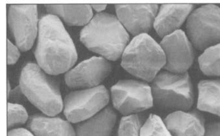
Polycrystalline boron nitride particles. (Photo courtesy of Hideo Ohara.)
