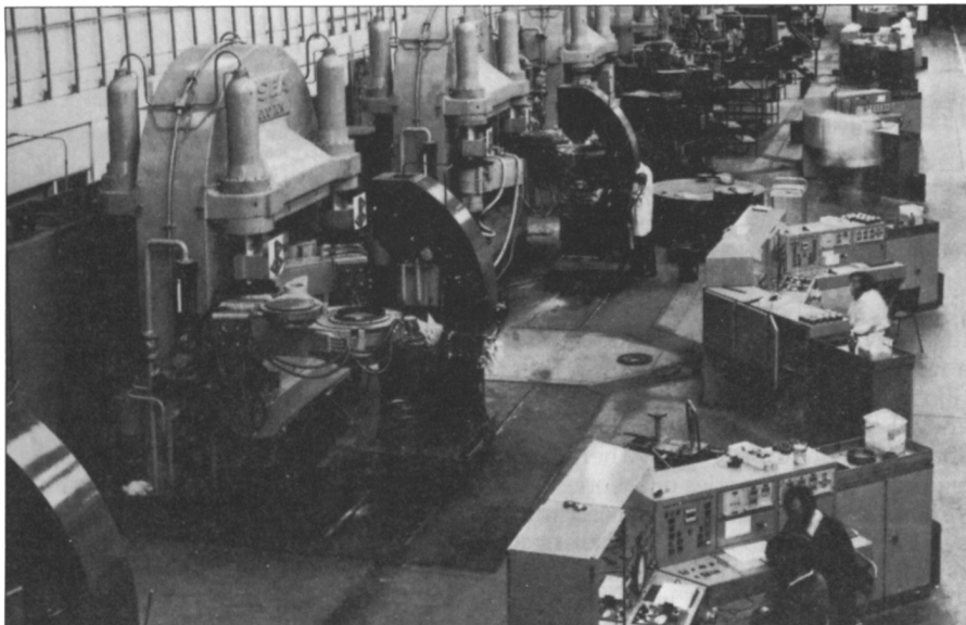
Figure 1. A diamond-manufacturing facility using the high-pressure, high-temperature (HPHT) process. Courtesy of DeBeers Industrial Diamond Division.
