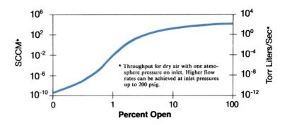
GPC Precision Leak Valves Provide Fourteen Decades of Smooth, Stable Flow Control.
