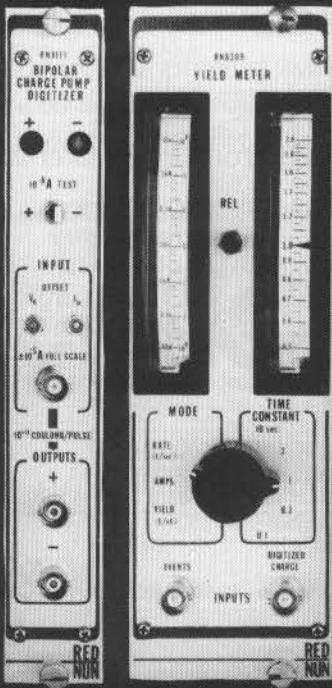
RN8111 — True bipolar response current integrator with 10 pico-Coulomb quantization spanning -10uA to +10uA. Features sensitivity and accuracy and no range switching.
