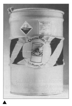
**Inflatable Spill-Control Device:** The DrumRoll<sup>®</sup> from ILC Dover can stop 55-gallon-drum leaks that are up to 7" x 2" in size. To stop a leak, users wrap the device around the drum and pull the inflation cord. A CO<sub>2</sub> cartridge then inflates a chemically resistant Teflon-coated bladder which stops the leak. No tipping or pegging is required, and one person may operate the device alone. A reusable training kit includes a DrumRoll<sup>®</sup> that can be
