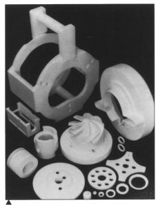
**Wet-Process Semiconductor Parts:** Engineering Plastics' EPI Wet Teflon® Process Semiconductor Parts are machined from a single piece of PTFE and PTFM with tolerances of 0.003 in. (~0.76 m). The parts provide less than 0.01% water absorption over 24 h and are unaffected by photoresists, acids, and corrosives. They can withstand from -450°F to +500°F (~ -265–257°C) operation, and can be rinsed with deionized water. Their low coefficient of friction virtually eliminates particle shedding.
