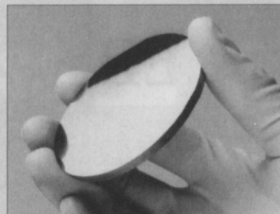
4000-MICRON THICK SILICON WAFER
