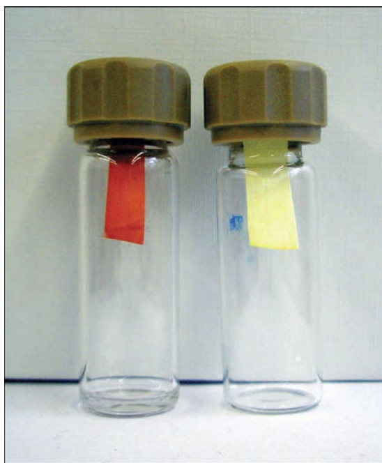
Figure 8. \text{HN}_3 can be detected by a filter paper impregnated with \text{FeCl}_3 . The color of the paper immediately turns into red upon contact with the headspace of the vial filled with \text{TMSN}_3 and MeOH (left vial; right vial is an empty vial for comparison) [44]
