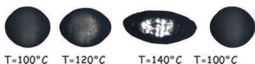
Figure 10. Optical micrographs of a 300- \mu\text{m} crosslinked liquid crystalline particle at different temperatures (adapted from ref. 22 )
