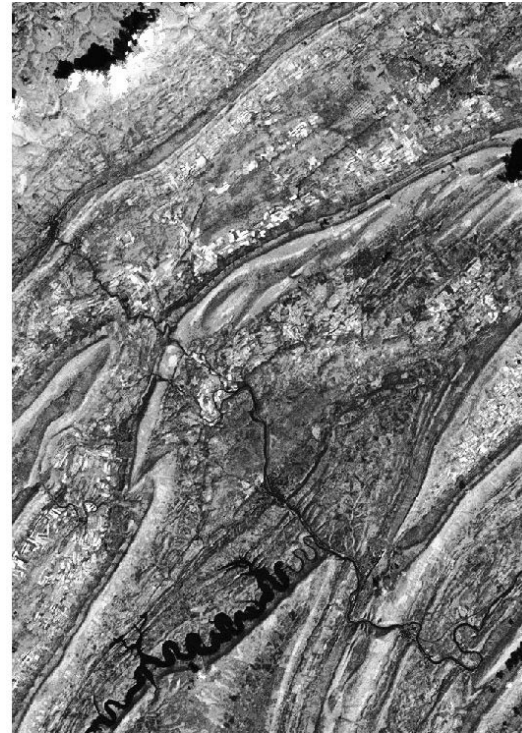
Figure 4. PHASE output of segmentation process for September 1991 sample of Landsat MSS image in central Pennsylvania.
