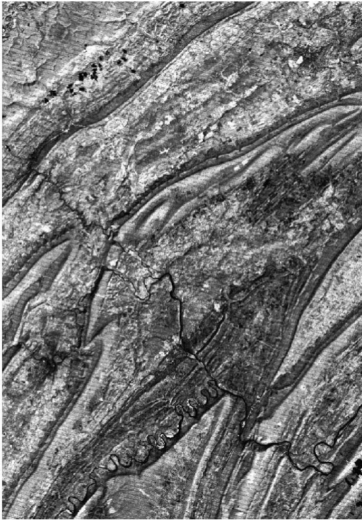
Figure 3. PHASE output of segmentation process for September 1972 sample of Landsat MSS image in central Pennsylvania.
