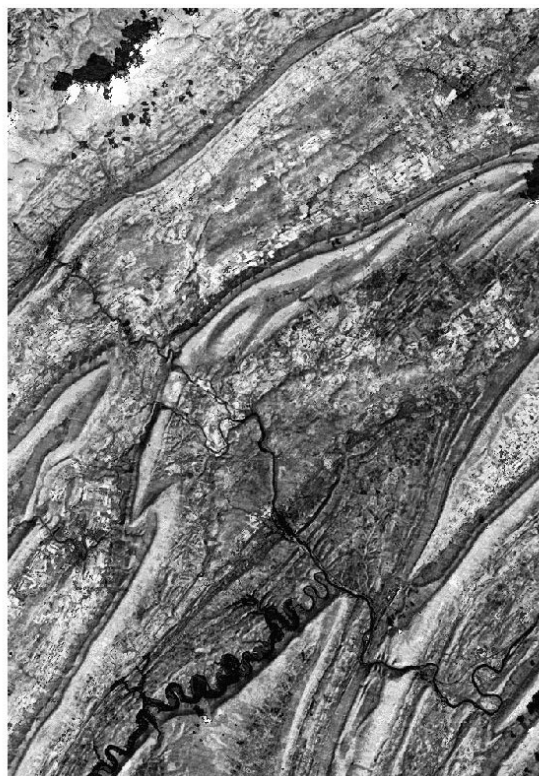
Figure 7. Grayscale rendering of PSI/PHASE conversion for multi-temporal composite of Landsat MSS subscenes from 1972 and 1991 in central Pennsylvania.
