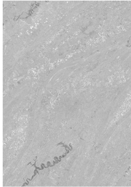
Figure 11. Image of scaled band 3 component of change as computed from Landsat MSS of central Pennsylvania from 1972 to 1991. Notice that the change for flooding of a reservoir is seen differently from changes in vegetative cover of land surface.
