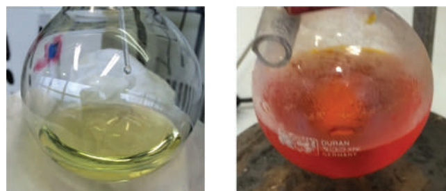
Figure 1. Comparison of crude reaction mixtures from flow (yellow) and batch (red) reactions
