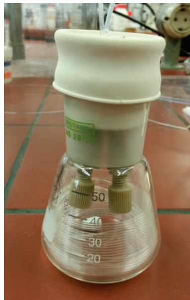
Figure 1. The “tube-in-flask” reactor consisted of a 50-mL standard Erlenmeyer flask in which 5 m of a Teflon AF-2400 tubing was coiled
