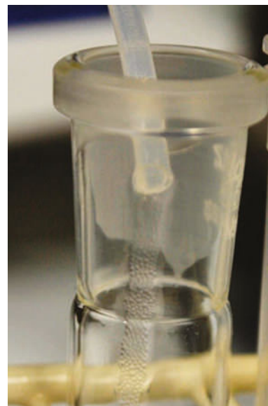
Figure 2. Microdroplets of n -heptane in an aqueous solution at the outlet from the PTFE tube connected with Corning LF module. Total flow rate, 0.8 mL/min; 25 ^{\circ}\text{C} ; 5 v/v% of added CaLB solution
