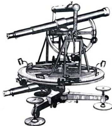
Fig. 4. Reichenbach's repetition theodolite for angular measurement
