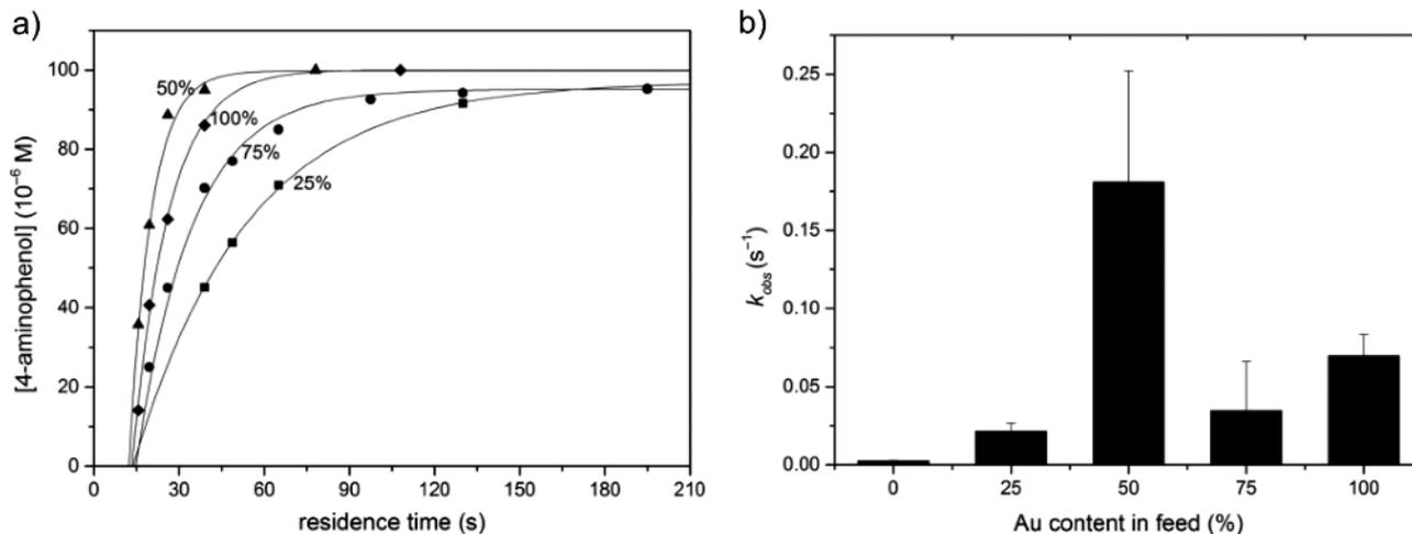
**Figure 3.** a) Formation of 4-aminophenol versus residence time in G4-NH<sub>2</sub> Au/Ag- and G4-NH<sub>2</sub> Au-functionalized microreactors for different gold contents in the metal feed (%). b) Observed rate constants versus nominal Au content (the error bars represent standard deviations of multiple measurements). [4-Nitrophenol] = 0.1 mM, [NaBH<sub>4</sub>] = 2 mM, water, rt
