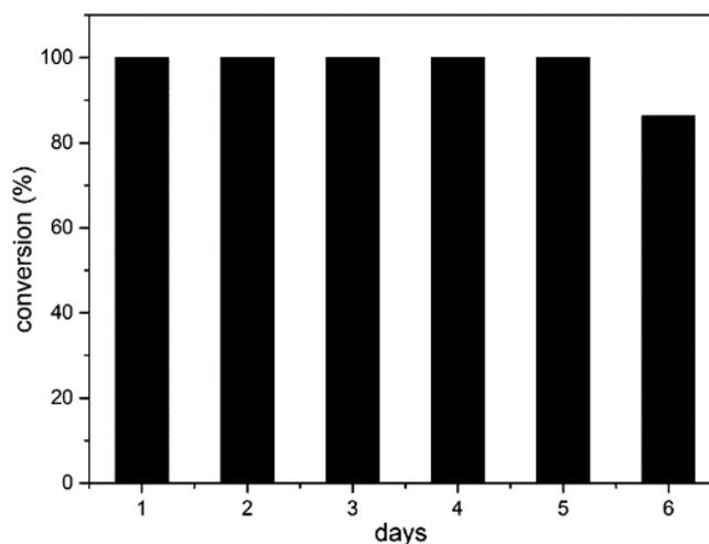
**Figure 4.** Conversion versus residence time for the reduction of 4-nitrophenol in a G4-NH<sub>2</sub> Au/Ag 1:1-functionalized microreactor. [4-Nitrophenol] = 0.1 mM, [NaBH<sub>4</sub>] = 2 mM, water, rt, residence time: 78 s
