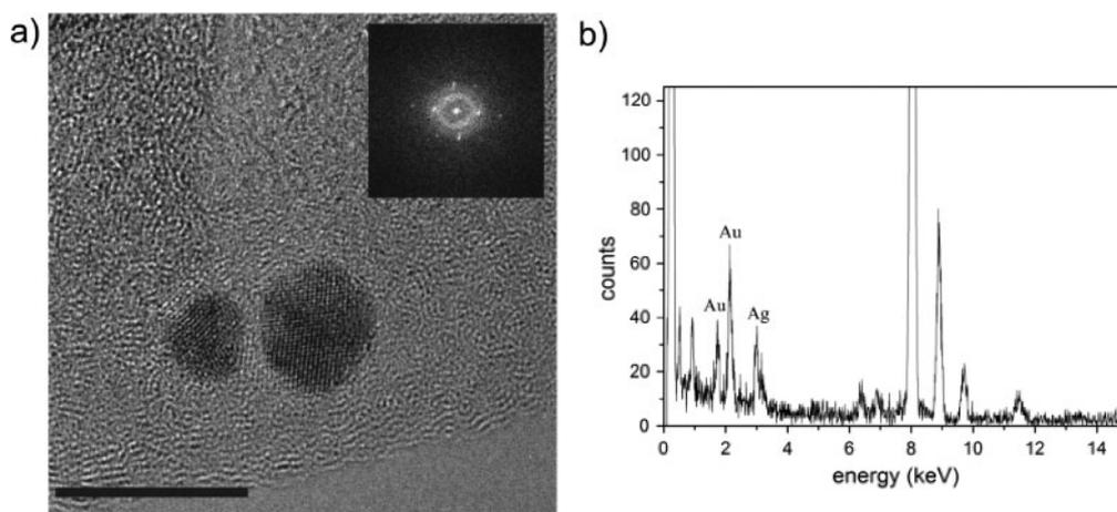
**Figure 2.** a) HRTEM image of a single crystal of a DEN Au/Ag 1:1 nanocomposite and a Fourier transformed image indicating the electron diffraction pattern in the inset (scale bar, 10 nm). b) EDX spectrum of the DEN Au/Ag 1:1 nanocomposite
