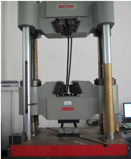
Fig. 2. The testing machine and resistivity detector: (a) loading apparatus, and (b) digital electrical instrument (SYSCAL-R2).
