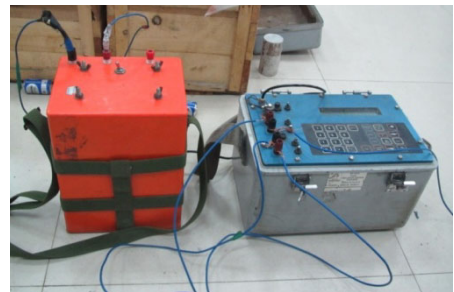
Fig. 2. The testing machine and resistivity detector: (a) loading apparatus, and (b) digital electrical instrument (SYSCAL-R2).
