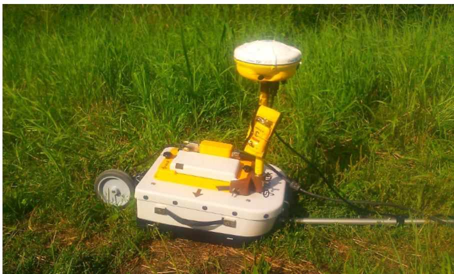
Fig. 3. Integrated survey set (ground penetrating radar antenna and GPS receiver).
