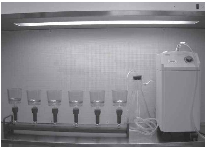
Fig. 2. Six-channel filtration system. Yeast cells in liquid medium are collected on the 47-mm water membranes contained in the funnels by the vacuum drawn from a pump (right).
