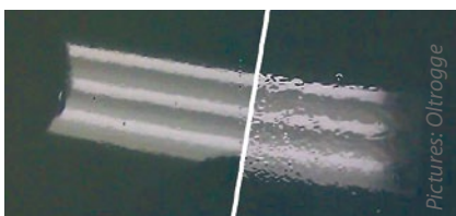
Nitrogen (left) versus compressed air (right): The picture on the left shows the first spraying attempt with the atomiser pressure reduced by half and without fine-tuning the application parameters. The coating applied was around 40% thicker.
