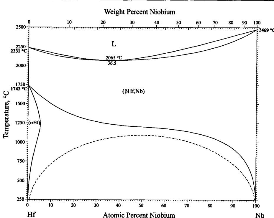
**Fig. 1** The Hf-Nb phase diagram.
