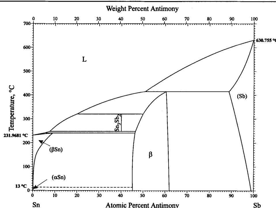
Fig. 1 The Sn-Sb phase diagram.
