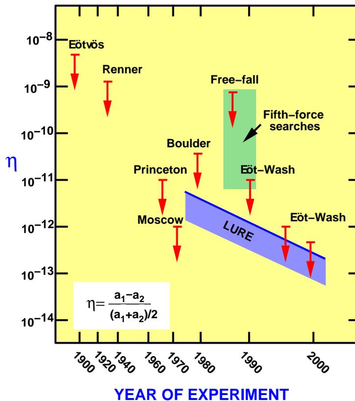
Figure 1: Selected tests of the weak equivalence principle, showing bounds on  $\eta$ , which measures fractional difference in acceleration of different materials or bodies. The free-fall and Eöt-Wash experiments were originally performed to search for a fifth force. The blue band shows current bounds on  $\eta$  for gravitating bodies from lunar laser ranging (LURE).
