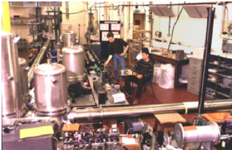
Figure 8: The 10 m prototype gravitational wave detector at Glasgow.
