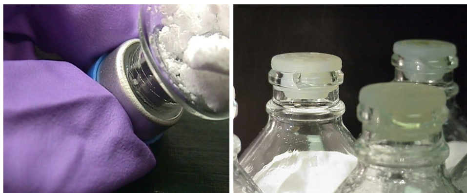
Fig. 10 Examples of vial damage resulting from excessive crimping pressure
