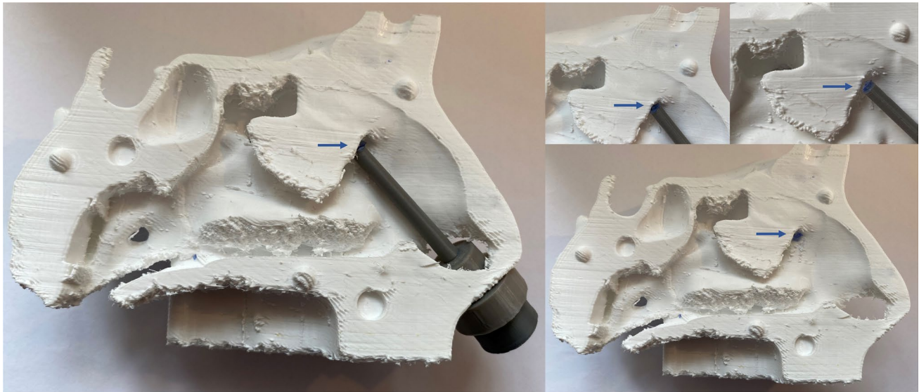
Fig. 5 Successful positioning of the nasal film (blue arrows) on the olfactory area of the semi-realistic nasal cast, using MPD
