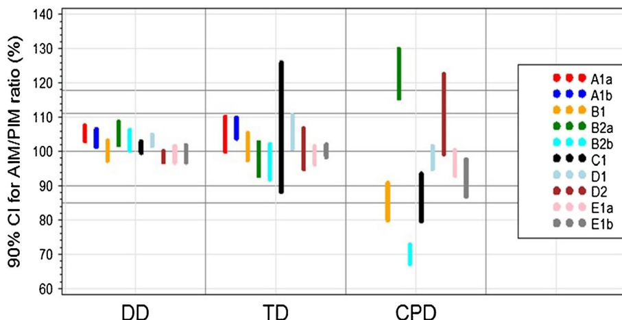
Fig. 7. 90% Confidence intervals for AIM/PIM ratio of secondary metrics DD, TD, and CPD for each product
