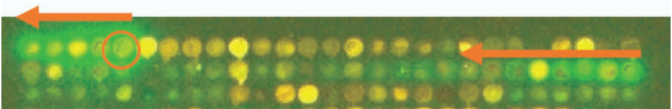
Figure 19. The print direction is right to left in successive rows moving down as illustrated with the arrows.
