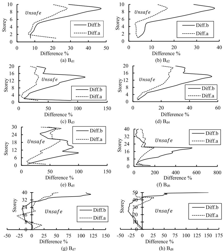
**Fig. 3** Differences in moment for horizontal members between OA and SAT before and after mitigation. **a** B<sub>d1</sub>, **b** B<sub>d2</sub>, **c** B<sub>d3</sub>, **d** B<sub>d4</sub>, **e** B<sub>d5</sub>, **f** B<sub>d6</sub>, **g** B<sub>d7</sub>, **h** B<sub>d8</sub>
