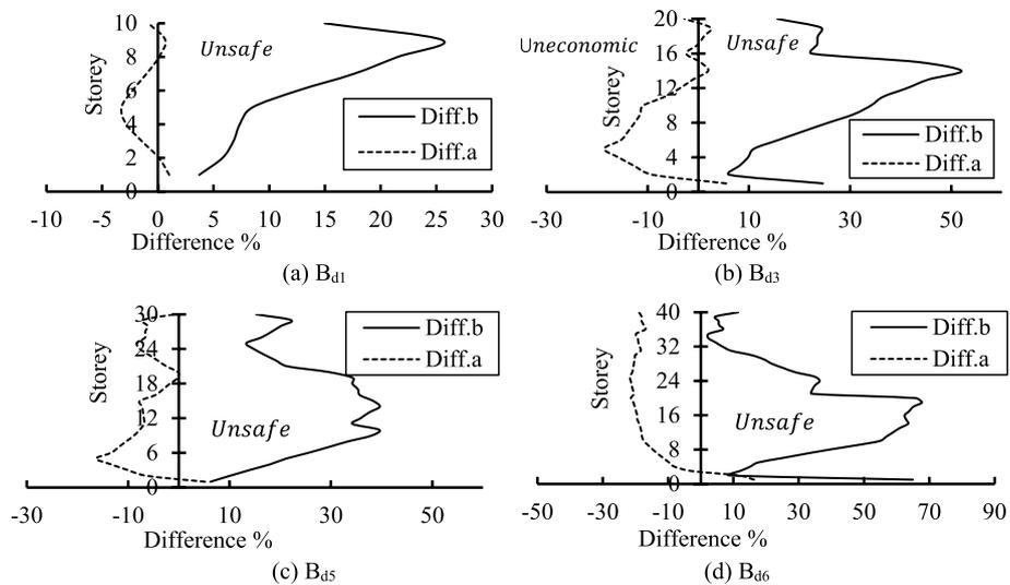
**Fig. 7** Differences in shearing force at beam ends between OA and SAT. **a** B<sub>d1</sub>. **b** B<sub>d3</sub>. **c** B<sub>d5</sub>. **d** B<sub>d6</sub>
