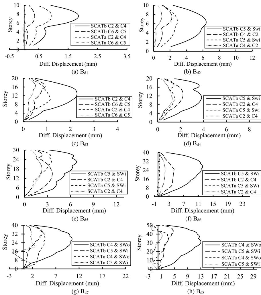
**Fig. 2** Differential displacement due to SATb and SATa. **a** B<sub>d1</sub>. **b** B<sub>d2</sub>. **c** B<sub>d3</sub>. **d** B<sub>d4</sub>. **e** B<sub>d5</sub>. **f** B<sub>d6</sub>. **g** B<sub>d7</sub>. **h** B<sub>d8</sub>
