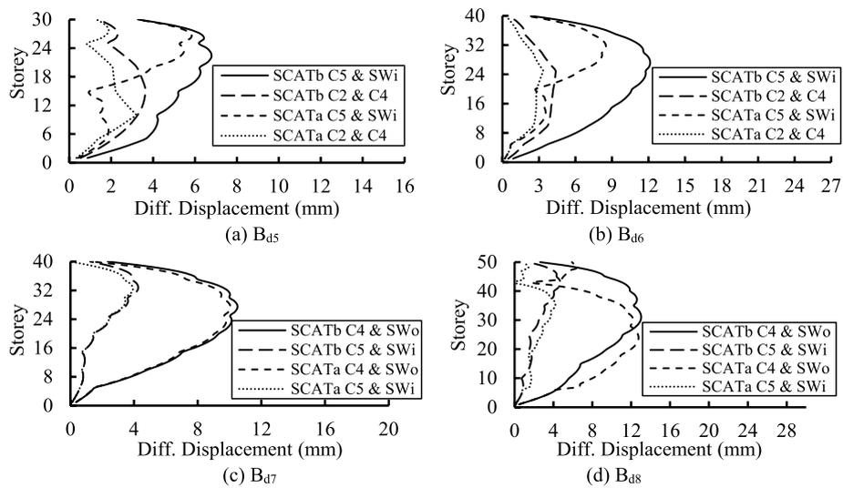
**Fig. 8** Differential displacement in members due to SATb and SATa. **a** B<sub>d5</sub>. **b** B<sub>d6</sub>. **c** B<sub>d7</sub>. **d** B<sub>d8</sub>
