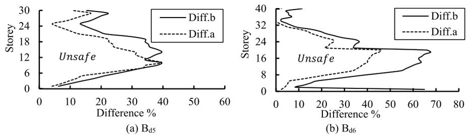
**Fig. 10** Deviations in moments for beams between SATb and SATa. **a**  $B_{d5}$ ; **b**  $B_{d6}$
