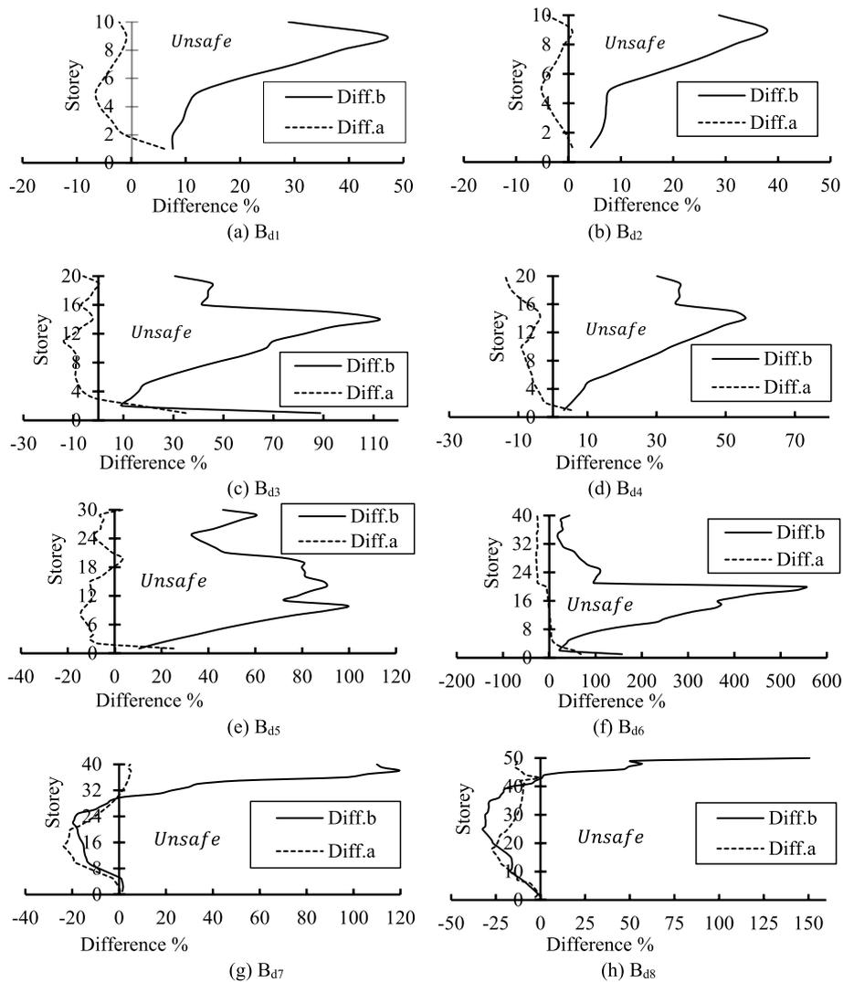
**Fig. 6** Differences in moments for horizontal members between OA and SAT. **a** B<sub>d1</sub>. **b** B<sub>d2</sub>. **c** B<sub>d3</sub>. **d** B<sub>d4</sub>. **e** B<sub>d5</sub>. **f** B<sub>d6</sub>. **g** B<sub>d7</sub>. **h** B<sub>d8</sub>
