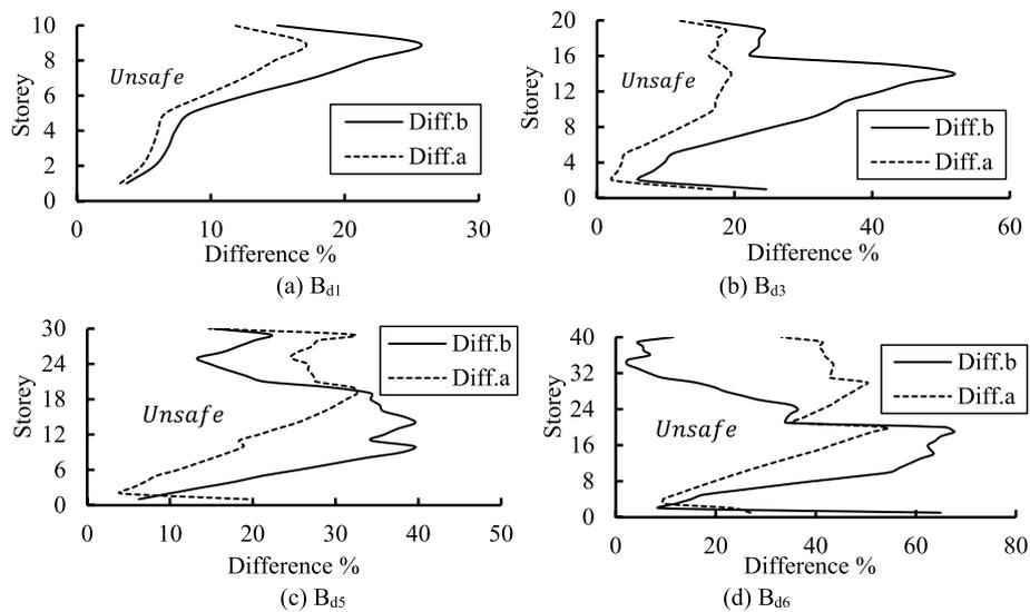
**Fig. 4** Differences in shearing forces at beam ends between OA and SAT. **a** B<sub>d1</sub>. **b** B<sub>d3</sub>. **c** B<sub>d5</sub>. **d** B<sub>d6</sub>
