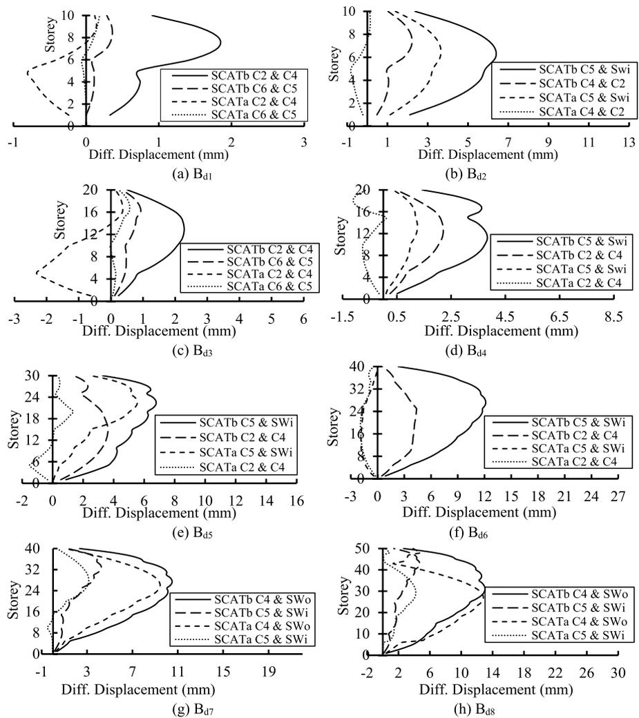
**Fig. 5** Differential displacement in investigated members due to SATa and SATb. **a** B<sub>d1</sub>, **b** B<sub>d2</sub>, **c** B<sub>d3</sub>, **d** B<sub>d4</sub>, **e** B<sub>d5</sub>, **f** B<sub>d6</sub>, **g** B<sub>d7</sub>, **h** B<sub>d8</sub>
