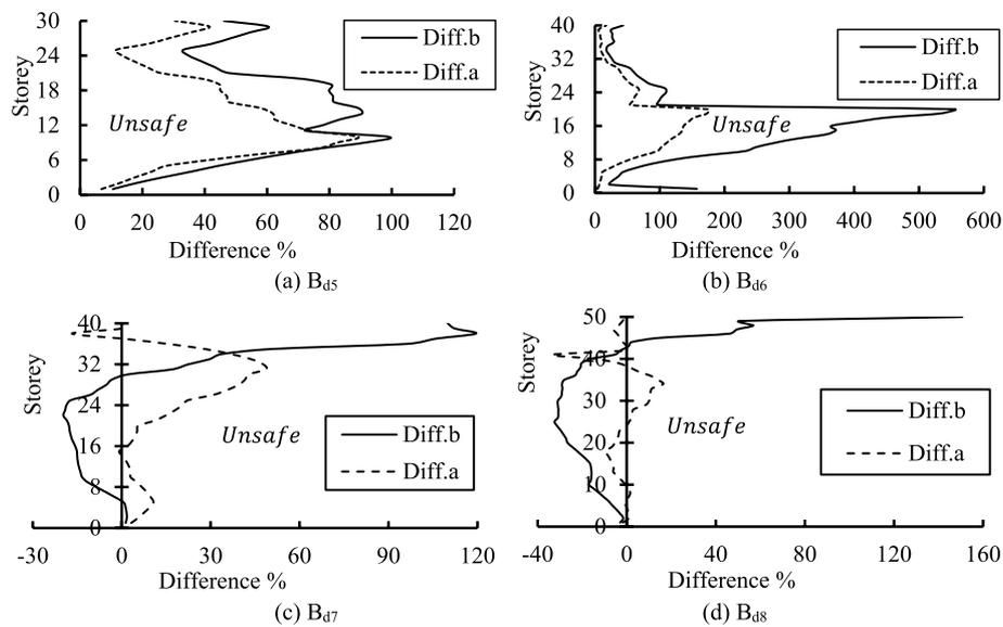
**Fig. 9** Deviations in moments for horizontal members between SATb and SATa. **a** B<sub>d5</sub>, **b** B<sub>d6</sub>, **c** B<sub>d7</sub>, **d** B<sub>d8</sub>
