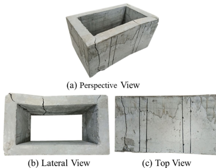
Fig. 14 Crack pattern for unconfinement specimen G02-S04-VUN
