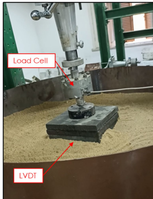
(a) Photo of the test rig
