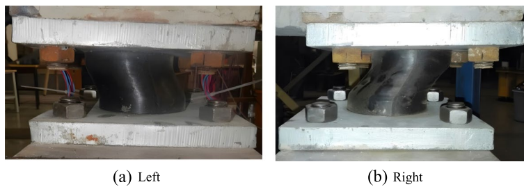
Fig. 10 Test deformation diagram of the bearing
